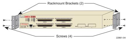
Figure 3-3 Installing the Rackmount Brackets
